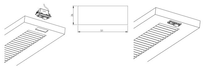
Ensure the face of the unit sits level with the luminaire casing and secure the unit in place.
