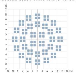
Detection range and sensitivity depends on the speed and size of the moving object as well as its temperature difference to the surroundings. Moving directionally towards the sensor will give worse detection than crossing the detection area on an angle.
