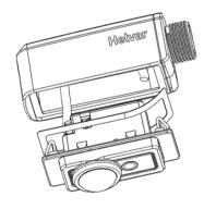
b) Remove the tape liner and feed the cable through the holder.
