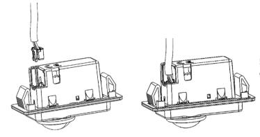
5636 Multisense High Bay has a connector for the Freedom connecting cable.
