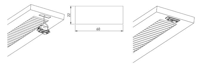
Carefully push the unit into the cutout until it 'clicks' into place and sits flush with the luminaire casing. Supported luminaire frame thickness in the range  $0.4 \le d \le 1.5$  mm.
