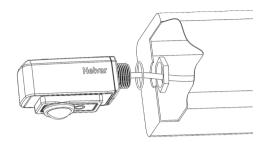
d) Feed the cable through the hole in the luminaire, connect the cable to the LED driver and fasten the holder to the luminaire using the O-ring and a M20 nut.
