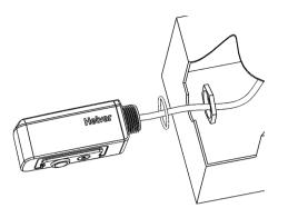
d) Feed the cable through the hole in the luminaire, connect the cable to the LED driver and fasten the holder to the luminaire using the 0-ring and a M20 nut.
