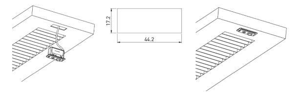
Carefully push the unit into the cutout until it 'clicks' into place and sits flush with the luminaire casing. Supported luminaire frame thickness in the range  $0.4 \le d \le 1.5$  mm.
