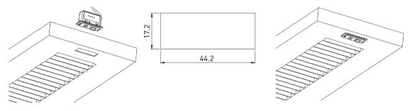
Ensure the face of the unit sits level with the luminaire casing and secure the unit in place.
