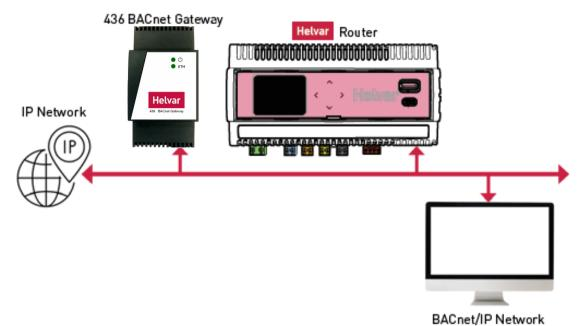
The BACnet Gateway allows a BMS to control and monitor the lighting system as well as obtain device status and group power consumption information. BACnet/IP clients can easily connect with the gateway via a TCP/IP network.
