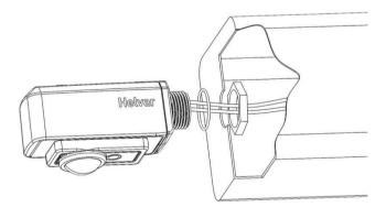
d) Feed the wires through the hole in the luminaire, connect them and fasten the holder to the luminaire using the 0-ring and a M20 nut.
