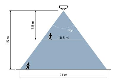
Detection pattern at floor level fot 15 m mounting height
