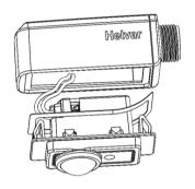
b) Remove the tape liner and feed the wires through the holder.
