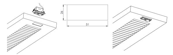
Ensure the face of the unit sits level with the luminaire casing and secure the unit in place.
