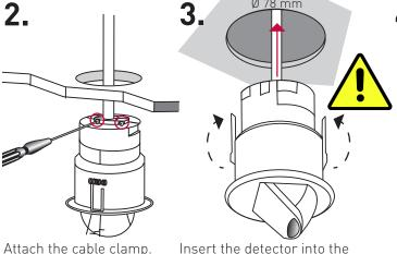
Attach the cable clamp.
