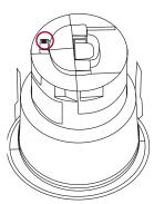
Carefully remove the metal locking clip, circled left, from rear of unit.
