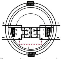
With some models, you must make a wire link between the DALI negative terminal and the negative terminal of the external power supply, as shown in the figure.
