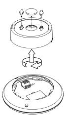
2. Thread the DALI cable through the housing mounting, and screw the housing mounting in place. Remove the DALI connector block from the receiver housing.
