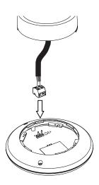
4. Re-attach the receiver housing (align with the housing mounting, insert and twist). Power on the DALI network.
